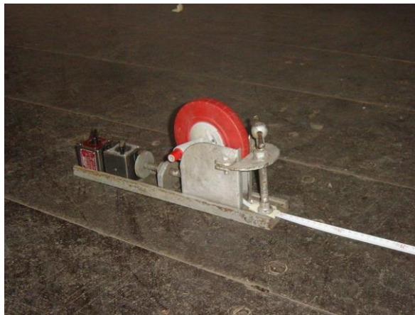
Figure 4-1: Arrangement for applying pull to measuring tape
